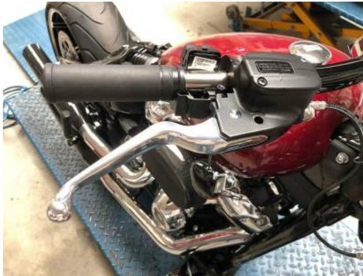
3. Pull indicator cables out as far as possible (push from center of handlebar).
